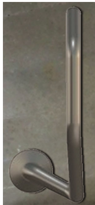
Fig. 5 — Modified silencer with 1 set of radial air injectors (8 radial jet injectors) placed at a distance of 100 mm from the silencer end.
